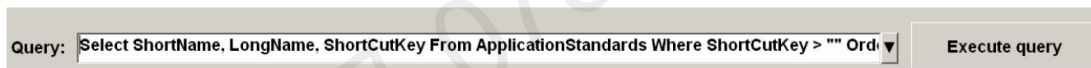
图 59: 输入以下指令: Select ShortName, LongName, ShortCutKey From ApplicationStandards Where ShortCutKey > "" Order By ShortName
