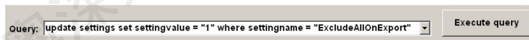
图 42: 在[Query]文本框中输入以下指令: update settings set settingvalue = “1” where settingname = “ExcludeAllOnExport”
